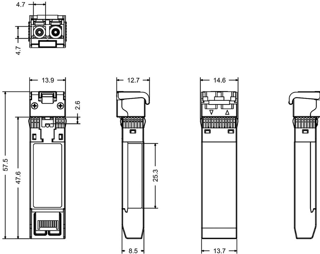
(All Dimensions are  $\pm 0.20\text{mm}$  Unless Otherwise Specified, Unit: mm)
